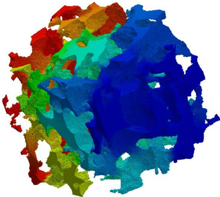
$$K_{ij} = \mu \langle v_i \rangle \left( \frac{\Delta P}{L} \right)^{-1} \quad i = x, y, z$$
